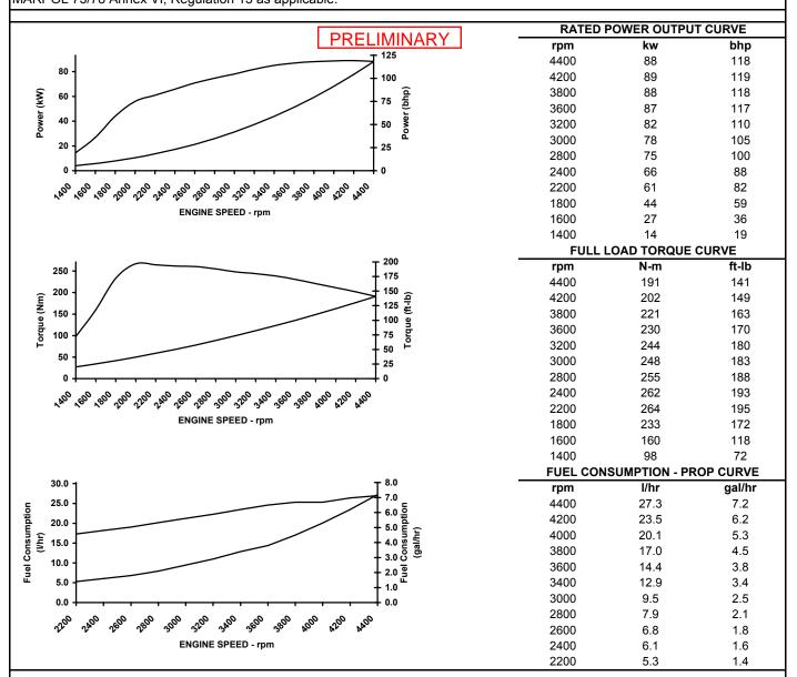
Rated Conditions: Ratings are based upon ISO 8665 and Sae J1228 referebce conditions; air pressure of 100 kPa [29.612 in Hg], air temperature 25deg. C [77 deg. F] and 30% relative humidy. Power is in accordance with IMCI procedure. Member NMMA
